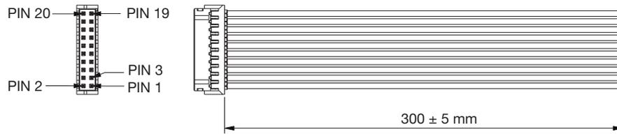
Order kit part number 73-788-001 for control connector interface with .3m wires attached
